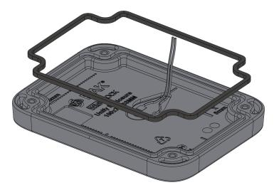
Figure 2: Installing the rubber gasket
