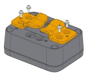
Figure 14: Fixing the pole mount on the enclosure
