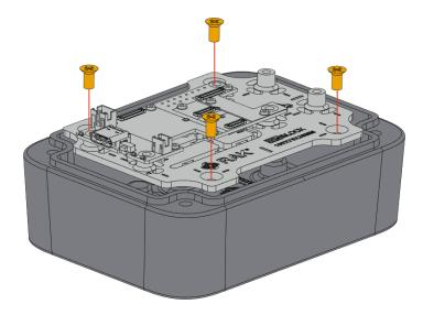
Figure 9: Installing Internal Mounting Plate to the enclosure
