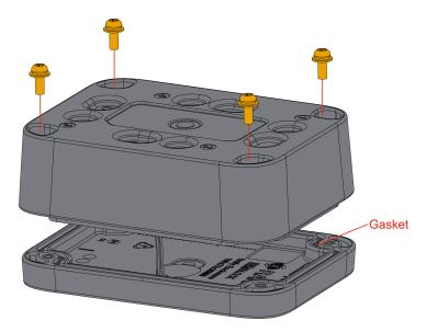
Figure 10: Closing the WisBlock Unify Enclosure
