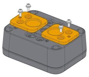
Figure 27: Fixing the magnet mount on the enclosure
