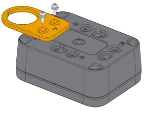
$\textbf{Figure 38:} \ \mathsf{Fixing the hook loop mount on the enclosure}$
