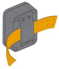
Figure 21: Fixing the enclosure on the belt clip
