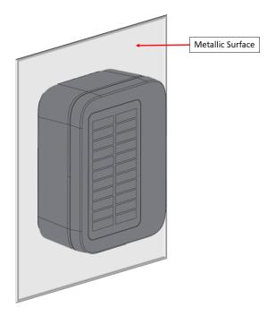
Figure 29: Fixing the enclosure onto the metal surface
