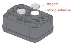
Figure 28: Fixing the magnet mount on the enclosure
