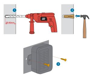
Figure 18: Fixing the enclosure on the wall
