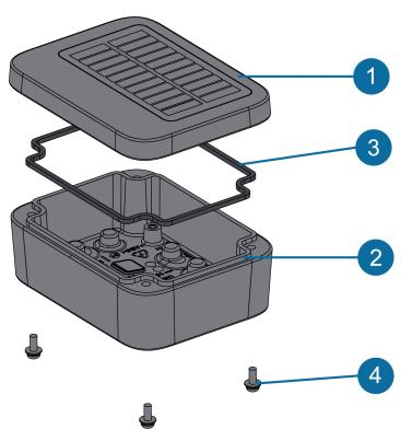
Figure 1: Small WisBlock Unify Enclosure package content
