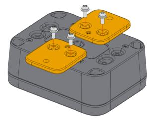
Figure 17: Fixing the wall mount on the enclosure
