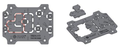
Figure 7: RAK19003 WisBlock Base board cut-out area
