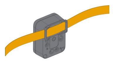
$\textbf{Figure 32:} \ \ \textbf{Fixing the enclosure on the belt thread}$
