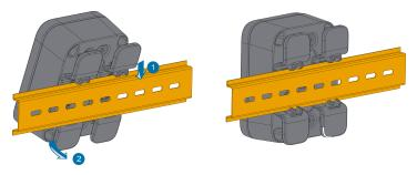
Figure 25: Fixing the enclosure on the DIN rail
