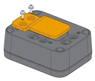
$\textbf{Figure 20:} \ \ \textbf{Fixing the belt clip mount on the enclosure}$
