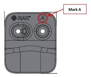
Figure 13: Mount accessory marked with letter A
