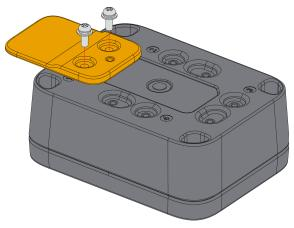
Figure 34: Fixing the label mount on the enclosure
