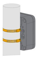
Figure 15: Fixing the enclosure on the pole
