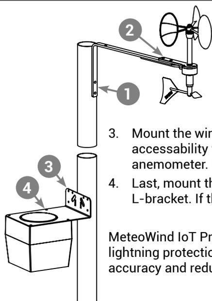
1. Mount the L-bracket onto a wall, fence, post, or mast, which will be used to support the anemometer. **Make sure it is pointing exactly North.**
