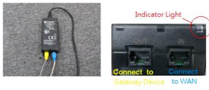
Figure 19 PoE Installation Instructions
