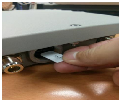
Figure 20 Sim card installation
