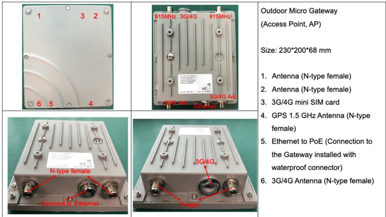
Figure 5 Gateway Installation Instructions
