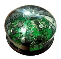
The GreenBox Tiny Zhaga is used for single control of streetlights.
