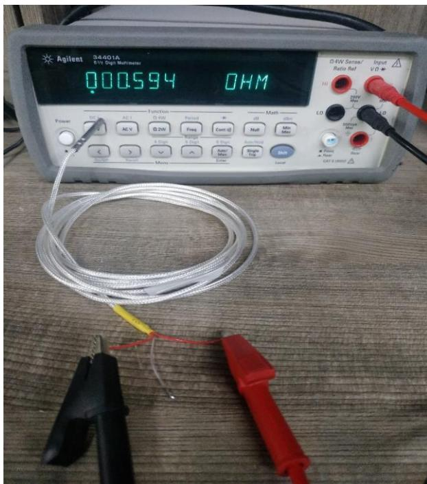
As example, in this step, we check the shorted wire (both red) with 0.594 ohm, So we know that each wire of PT100 has  $(0.594 - 0.002)/2 = 0.296\Omega$  (Where 0.002 is the value we got from step 1) .
