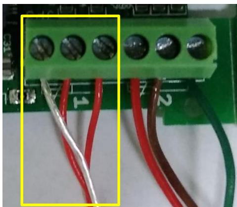
For a 3 wire PT100, there are two wire are shortcut, for example, as per above photo Channel 1, there are two red wire , which are shortcut in PT100, connect them as the photo. The 3<sup>rd</sup> wire (white wire ) connect to the left pin of Channel -1.
