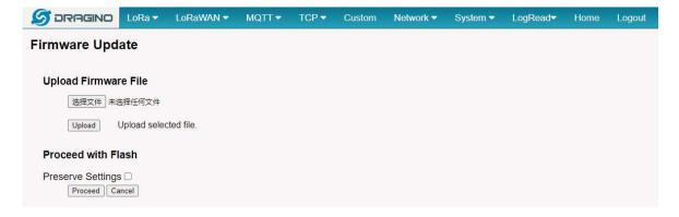
Select the required image and click Flash Image. The image will be uploaded to the device, and then click Process Update to upgrade.
