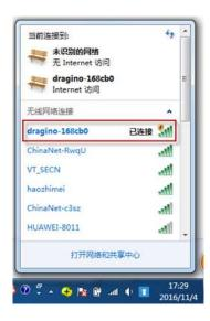
User can use a PC to connect to this WiFi network. The PC will get an IP address 10.130.1.xxx and the LG308N has the default IP 10.130.1.1
