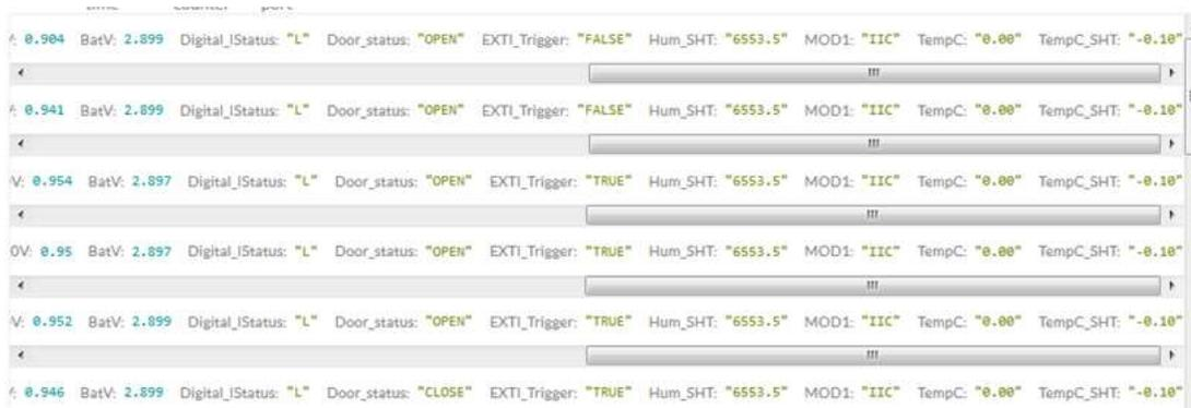
In **MOD=1**, user can use byte 6 to see the status for door open or close. TTN V3 decoder is as below:
