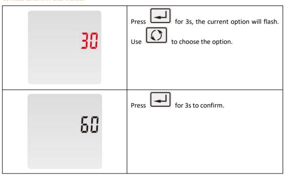
**NOTE:** Under the active upload mode, the OFF Line time should be set to a value bigger than the active upload interval time.
