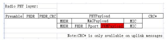
The following description of the text is defined the data in the segment of FRMPayload region in LoRaWAN protocol. The software in PC only need to get this part of data from gateway. According to the following protocol definition to parse the data.
