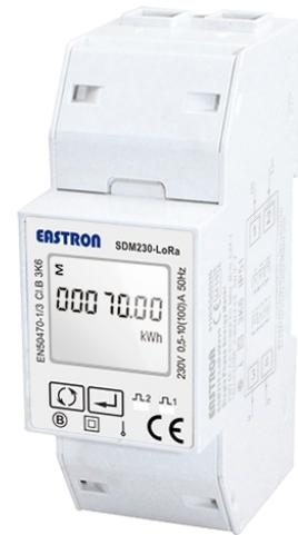
SDM230-Lora measures and displays the characteristics of single phase two wire(1p2w) supplies, including kWh, kVAh, kW, kVAR, kVA, PF, Frequency, Voltage, Current, dmd, THD etc. It support Max.100A direct connection, saving the cost to install external CTs. Maximum demand current can be measured over preset periods of up to 60 minutes. This unit has a built-in LoRaWAN module which allows long range wireless communication. Two pulse outputs are available for real time energy measurement.
