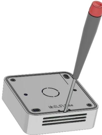
2. Install the batteries. The ERS CO<sub>2</sub> requires one or two AA batteries. The battery type is 3.6V Lithium Battery (ER14505). You can use one battery, but it's recommended that you use two for best performance and battery life. Use battery slot A if only one battery is used.
