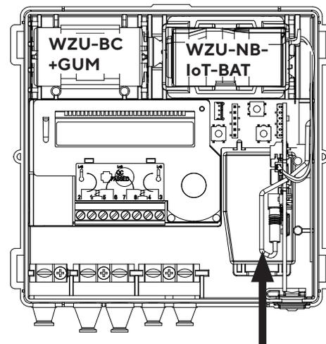
Cable routing internal antenna\*
