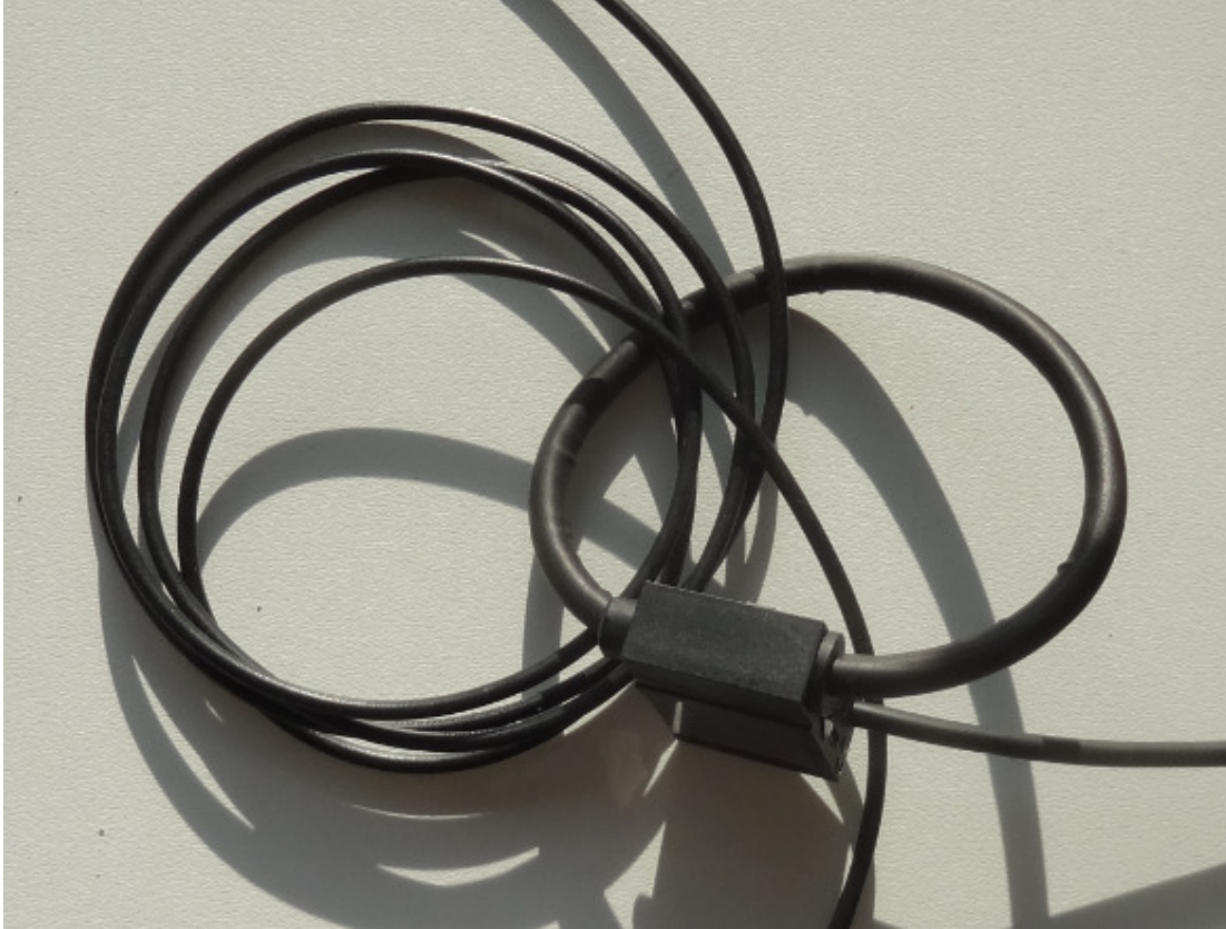
Figure 6-3 Sensitivity is 5 times higher if the power cable is wrapped around the coil 5 times
