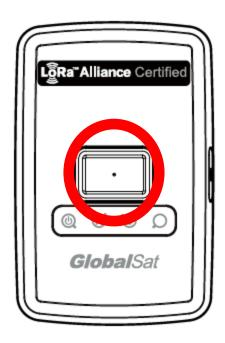
When help button is long pressed, LT-100 will send the first help report immediately. Then LT-100 would send help reports every 30 seconds (default value) continuously to  $LoRaWAN^{TM}$  gateway till it gets server acknowledgement and GPS fix.
