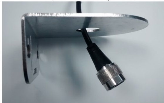
Figure 107 : N connector introduced in the hole of the dome antenna bracket
