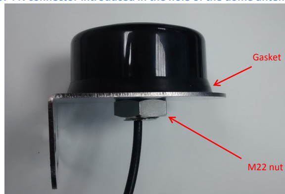
Figure 108 : Antenna installed on the dome antenna bracket
