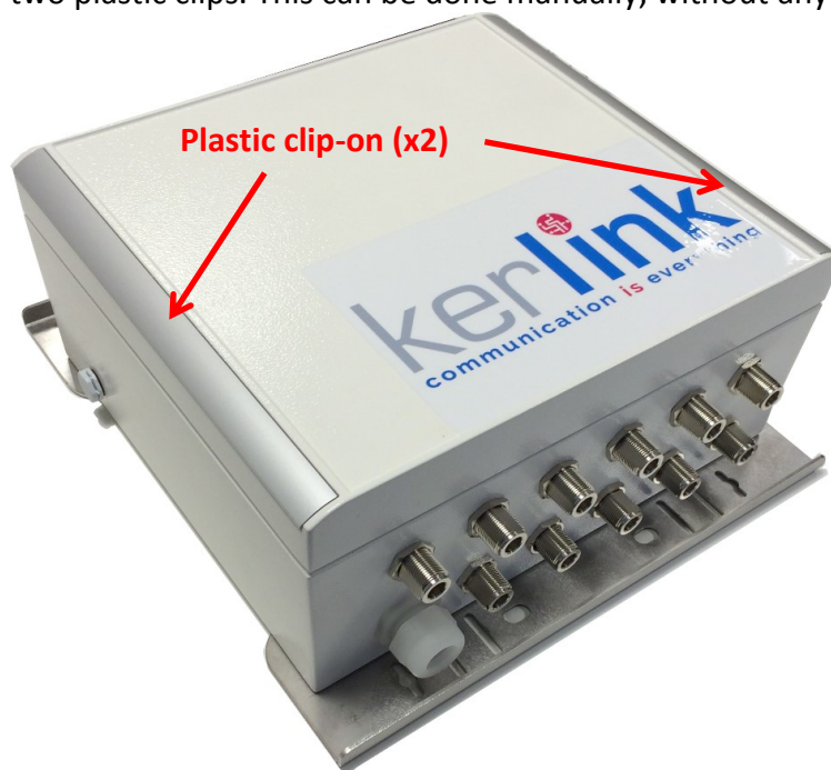
Figure 94: Wirnet iBTS – plastic clips on the lid
