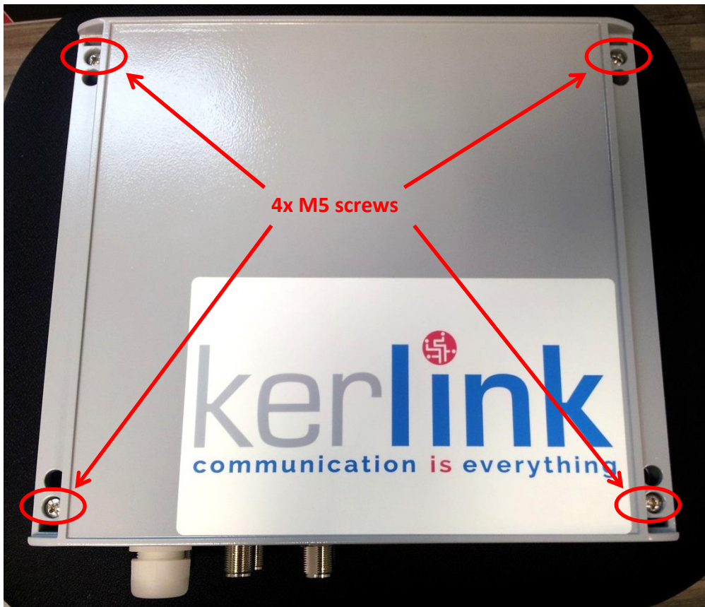
Figure 95: Wirnet iBTS – 4x M5 screws
