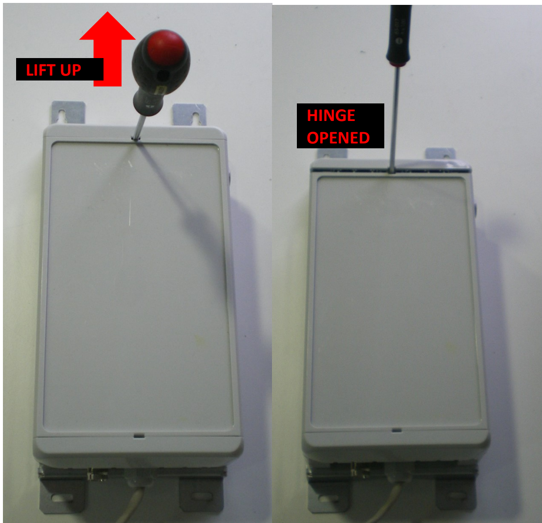
Figure 97 : Opening of the compact enclosure with screwdriver
