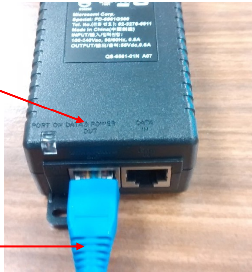
Figure 157 : Ethernet connection on PoE injector side
