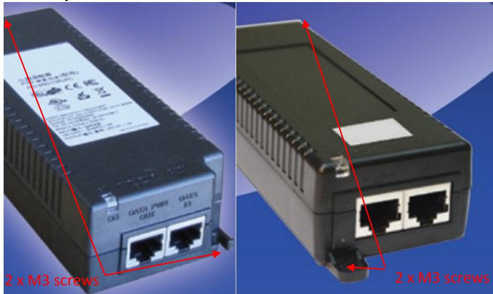
Figure 120 : Screws for indoor POE injectors mounting
