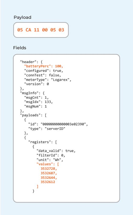
The screenshot shows the 'Payload' section of the The Things Network Backend. The payload is displayed as a hex string: `05 CA 11 00 05 03`. Below it, the 'Fields' section shows the decoded JSON data:
