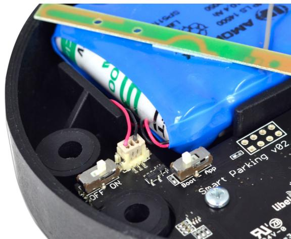
Figure : Smart Parking node "user switches"
