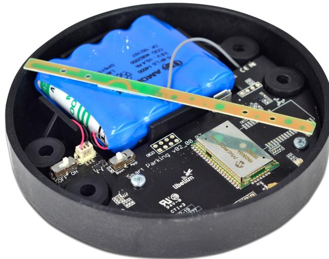
*Figure : Base of a Smart Parking node*
