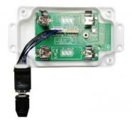
The USB adapter uses a six-wire JST-ZH series connector for attaching to Lobaro hardware at the config connector.
