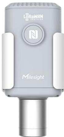
EM500-CO<sub>2</sub> is designed for measuring CO<sub>2</sub>, temperature, humidity and barometric pressure in harsh environments and transmitting data using LoRaWAN® technology. With this low power consumption technology, EM500-CO<sub>2</sub> can work up to 10 years with 19000 mAh battery. Combining with Milesight LoRaWAN® gateway and Milesight IoT Cloud solution, users can manage all sensor data remotely and visually.
