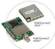
The mDot and xDot are LoRaWAN compliant, providing bi-directional data communication up to 10 miles line-of-sight and 2-3 miles in buildings, using the global sub-GHz ISM radio bands in North America, Europe, and the APAC regions.
