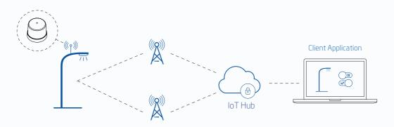
Luminaire controlling solution enables remote lighting control for LED or HID luminaires with DALI or using analog 0..10V. With better control over lighting you are able to reduce energy consumption, CO2 emission as well as allow efficient maintenance cycles.
