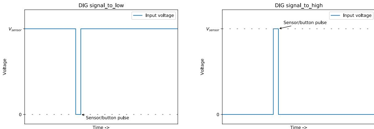
\*  $V_{sensor}$  is Device specific. For event to be registered, pulse duration must be at least 100ms.
