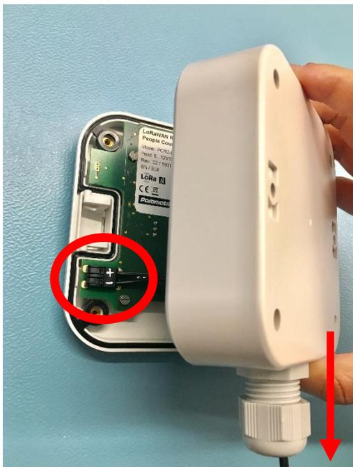
Before closing the casing, make sure that the two components are aligned as depicted:
