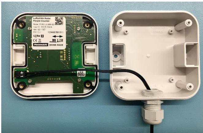
Guide the cable through the cable gland.
