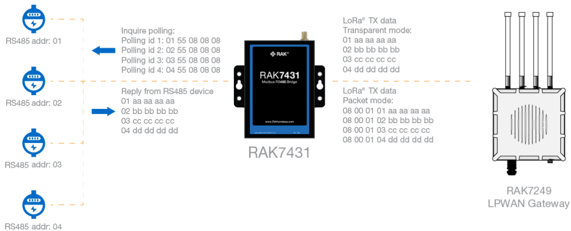
Figure 2: RAK7431 WisNode Bridge Serial polling mode
