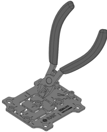
Figure 4: Cutting-out excess parts of the WisBlock Internal mounting plate
