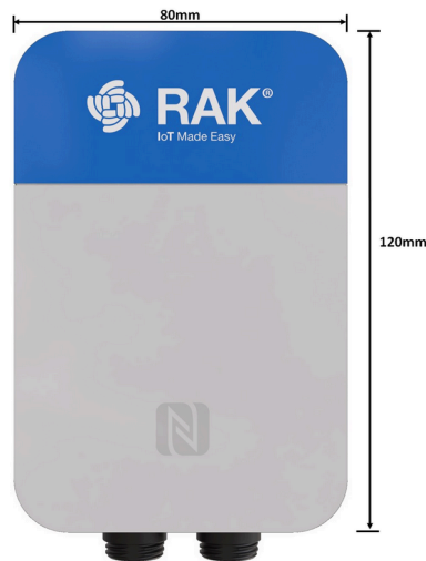
Figure 1: RAK2560 WisNode Sensor Hub dimensions
