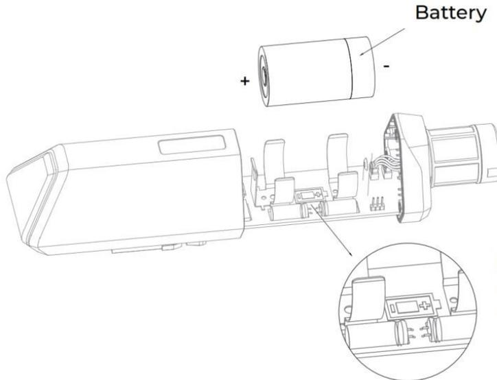
**Note:** Do not invert the positive and negative batteries. Otherwise, short circuit may occur and the device may be damaged.
