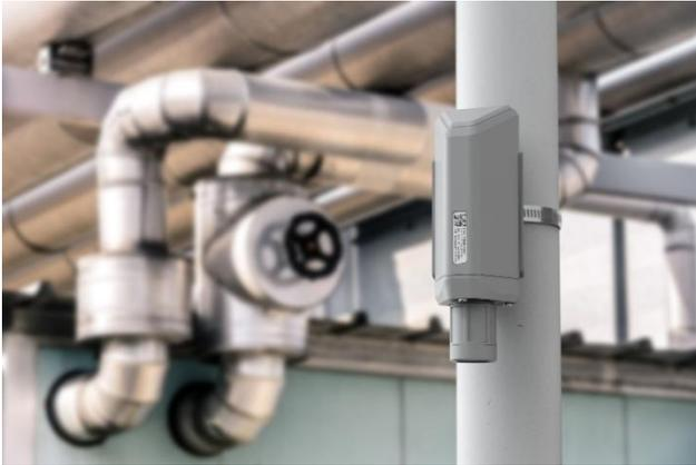
If the device is installed outdoors, it is important to avoid direct sunlight as it can cause thermal effects and result in higher temperature readings. To ensure more accurate measurements:
