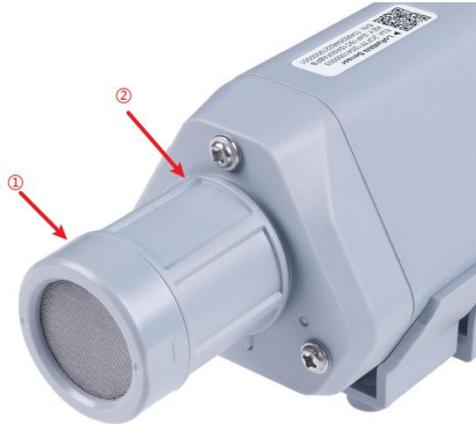
2. Do not open the inside of the sensor unless the battery needs to be replaced. This may result in abnormal waterproofing. If it is opened, make sure the waterproofing gasket is properly installed and tighten the screws.
