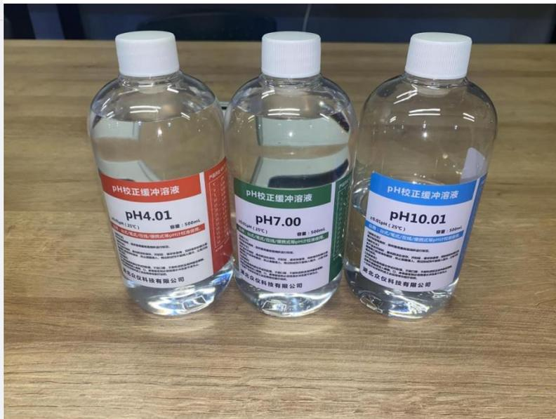
2) Prepare the standard liquid and pour an appropriate amount of the liquid into the graduated cylinder. Insert the pH probe electrode into the liquid in the graduated cylinder.
