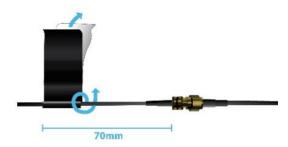
Keep the tape stretched while wrapping, over-lapping half the width of the previous turn.
