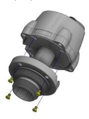
**Note:** This adaptor can also be used with the waveguide option but will require a 36mm pipe. The waveguide pipe should be securely attached via the two grub screws provided and hand tightened with an M1.5 Allen key (Note: over-tightening the grub screws can damage the plastic).
