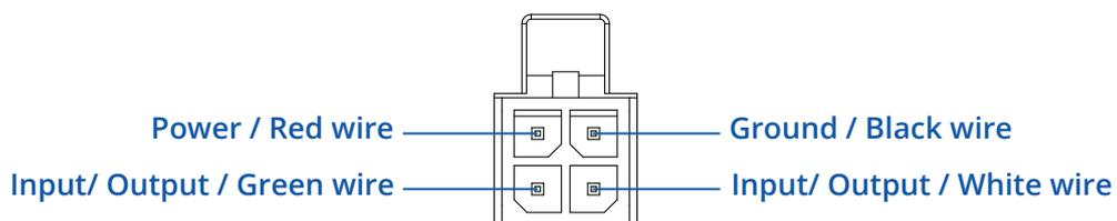
\*I/O: programmable Input/Output pins (Open Collector output max 30 V, 300 mA or Digital input where 0-6 V detected as logic low and 8-30 V - logic high).
