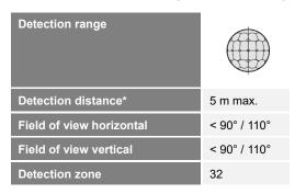
An detection distance of 2,5 m results in a square detection zone of approx. 5 x 5 m, or a circular detection zone of approx. Ø 7 m divided in 32 measuring zones.
