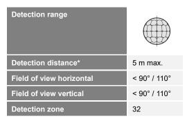
An detection distance of 2,5 m results in a square detection zone of approx. 5 x 5 m, or a circular detection zone of approx. Ø 7 m divided in 32 measuring zones.
