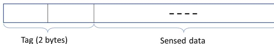
**Figure 1-8: Tagged LoRaWAN Frame Payload**
