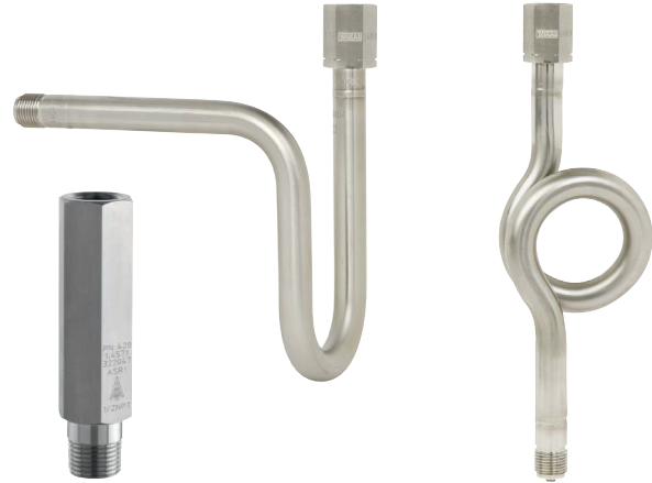
Wassersackrohre, Typ 910.15, CrNi-Stahl Abb. links: Kompaktform Abb. Mitte: U-Form, DIN 16282 Form A Abb. rechts: Kreisform, DIN 16282 Form C
