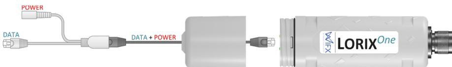
PoE Ethernet port supports 24VDC. Use only the provided power supply adapter. The max consumption is 3W.
