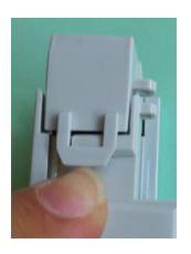
1. Open the sensor's movable jaw by lifting the tab on the side of the sensor.
