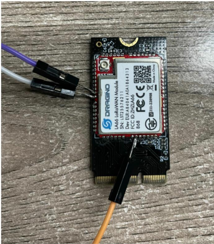
3. Connect JLINK, and switch mother board SW1 to ISP. Wire connection as below:
