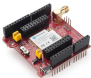
**LA66 LoRaWAN Shield** is the Arduino shield base on LA66. Users can use LA66 LoRaWAN Shield to rapidly add LoRaWAN or peer-to-peer LoRa wireless function to A
