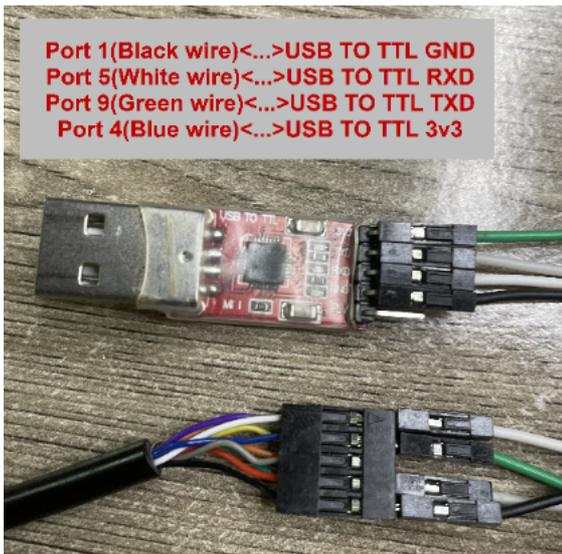
Then use DuPont cable to short circuit port3 and port1, and then release them, so that the device enters bootload mode.
