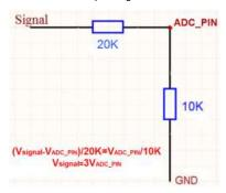
When ADC\_IN1 pin is connected to GND or suspended, ADC value is 0
