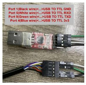
Then use DuPont cable to short circuit port3 and port1, and then release them, so that the device enters bootlaod mode.
