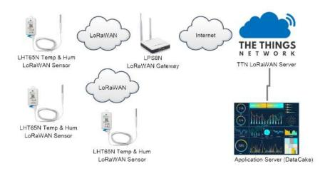
Assume the LPS8N is already set to connect to TTN V3 network (https://eu1.cloud.thethings.network) , So it provides network coverage for LHT65N. Next we need to at the LHT65N device in TTN V3:
