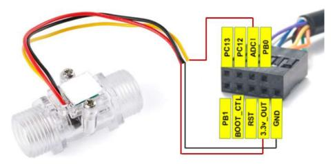
Case 2: Normal Flow Sensor: Such flow sensor has higher power consumption and is not suitable to be powered by LHT65N. It is powered by external power and output <3.3v pulse
