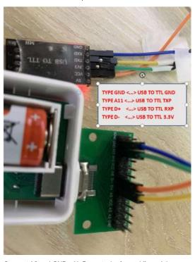
Connect A8 and GND with Dupont wire for a while and then separate ,  $\,$  enter reset mode
