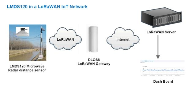
In this user case, the LMDS120 is installed on top of river to detect the water level and send the level info to
