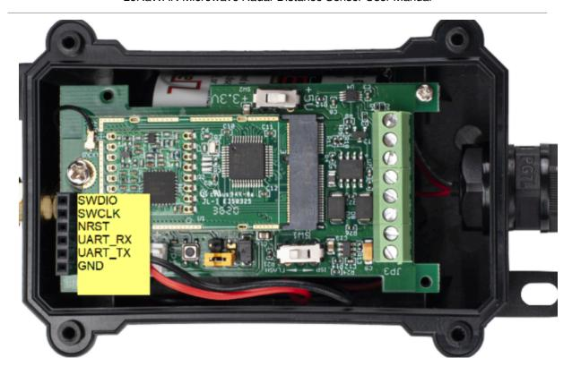
LMDS120 supports AT Command set. User can use a USB to TTL adapter plus the 3.5mm Program Cable to connect to LMDS120 to use AT command, as below.
