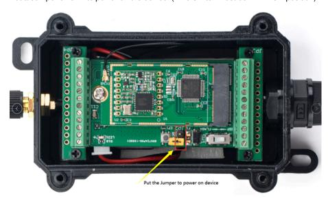
Put the jumper to power on LMDS120 and it will auto-join to the TTN V3 network. After join success, it will start to upload sensor data to TTN V3 and the user can see it in the panel.
