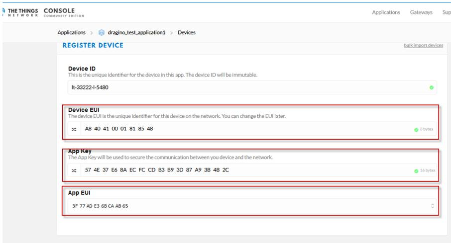
**Step 2:** Power on LT and it will auto join to the TTN network. After join success, it will start to upload message to TTN and user can see in the panel.
