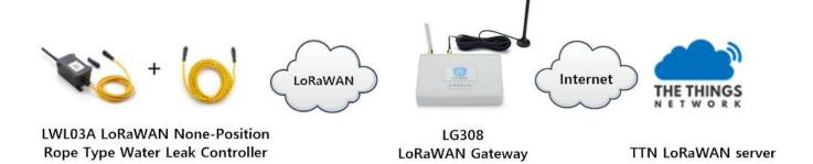
The LWL03A has water leak detect probe as above. When there is water between these two detect probe, they will be short and generate the water leak event. and send LWL03A will uplink two type of messages to the server.
