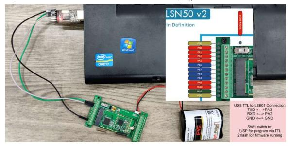
In the PC, you need to set the serial baud rate to 9600 to access the serial console for LWL03A. LWL03A will output system info once power on as below:
