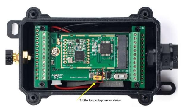
Put the jumper to power on LWL03A and it will auto-join to the TTN V3 network. After join success, it will start to upload sensor data to TTN V3 and the user can see it in t
