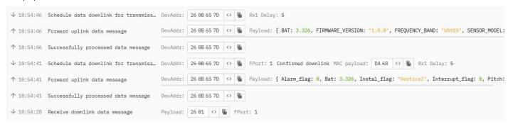
**Sensor Model**: For TS01-LB, this value is 0x2F **Firmware Version**: 0x0100, Means: v1.0.0 version
