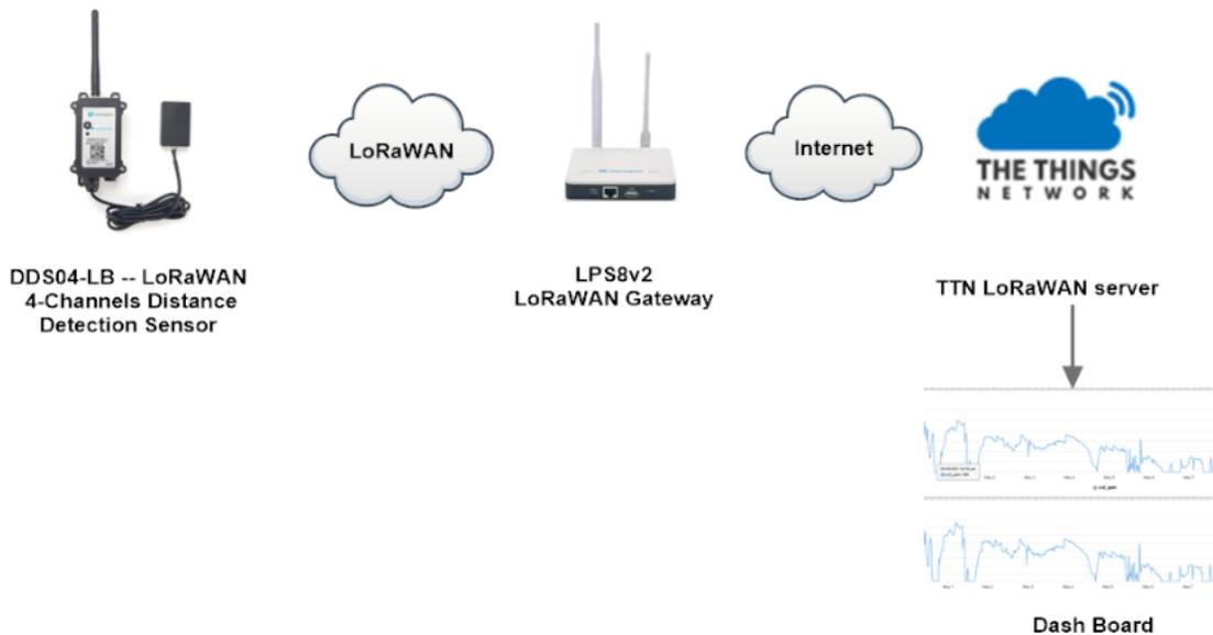
**Step 1:** Create a device in TTN with the OTAA keys from DDS04-LB.
