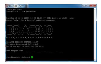
The "logread -f" command can be used to debug how system runs.
