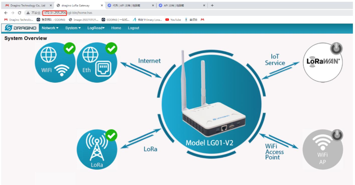
**Method 3:** Connect via WiFi with DHCP IP from the router
