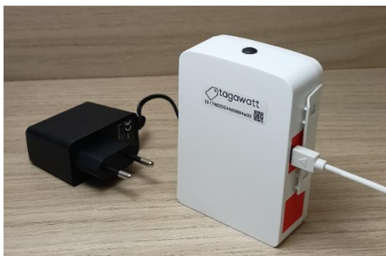
Fig. 9 – watt-L with a 5V adapter and the first wire of the chain
