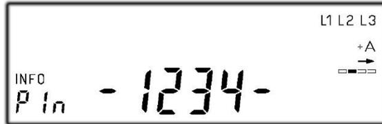
If the PIN is correct, the display then shows the performance
