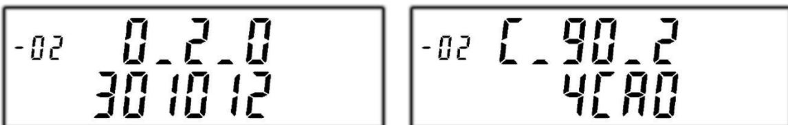
Rolling display of billing-relevant values. The display of the instantaneous power in the second line must be enabled by entering a PIN:
