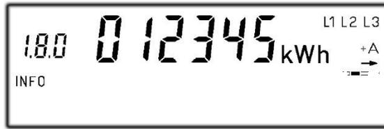
Double tariff variant for current direction + A: alternating display between registers 1.8.1 and 1.8.2
