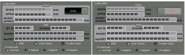
LoRa communication is protected with 2 AES keys. First, the user data (meter readings, etc.) are encrypted with an AppSKey. This data is supplemented by the communication layer of the LoRa-WAN and then all encrypted together with the NetSKey. This enables a separation between communication in the network and processing of the user data. For this purpose, the LoRa server forwards the encrypted user data to the application server, which in turn is able to decrypt and process this data.
