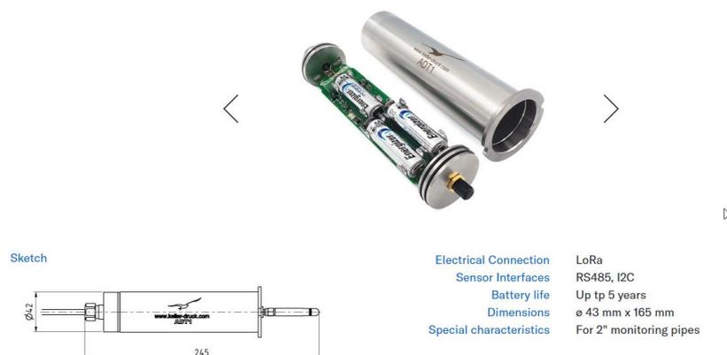
The remote data transmission unit ADT1-Tube is encased in a robust, stainless steel housing, which is ideally suited to installation in 2" monitoring pipes.
