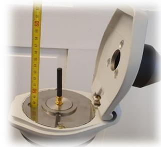
Connect the ADT1 device to the PC. To get access to the internal USB interface the ADT1 device must be opened.
